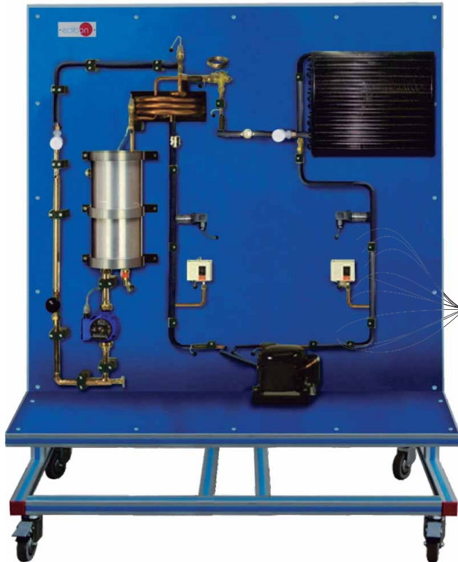
① Unit: TRCAC. Unit for the study of a Refrigeration Circuit with Variable Load
